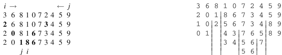
Fig. 5.8. Execution of qSort (Fig. 5.7) on \langle 3, 6, 8, 1, 0, 7, 2, 4, 5, 9 \rangle using the first element as the pivot and n_0 = 1 . The left-hand side illustrates the first partitioning step, showing elements in bold that have just been swapped. The right-hand side shows the result of the recursive partitioning operations
